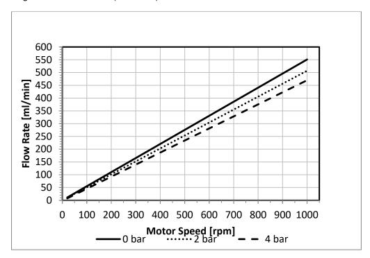
The flow rates showing at the chart above were ascertained with a new pump chamber under standard conditions after the final assembly of the pump.
