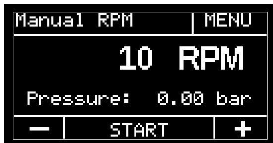
Picture 26 PendoTECH successful zeroing
